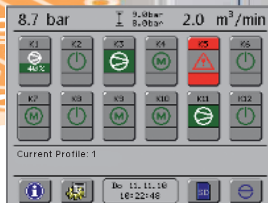
Compressor module (STD) for alternative compressors with fixed speed and/or half-/full-load control
